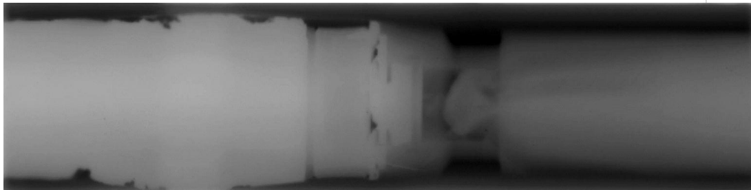
Neutron radiograph of irradiated FBTR Control rod
